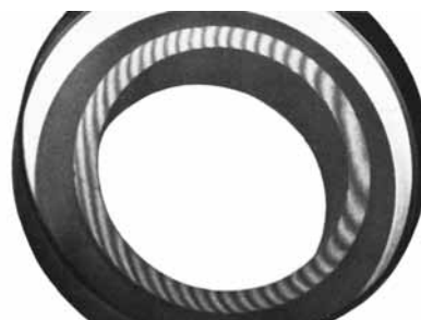
Sliding surface with imperfect flatness
